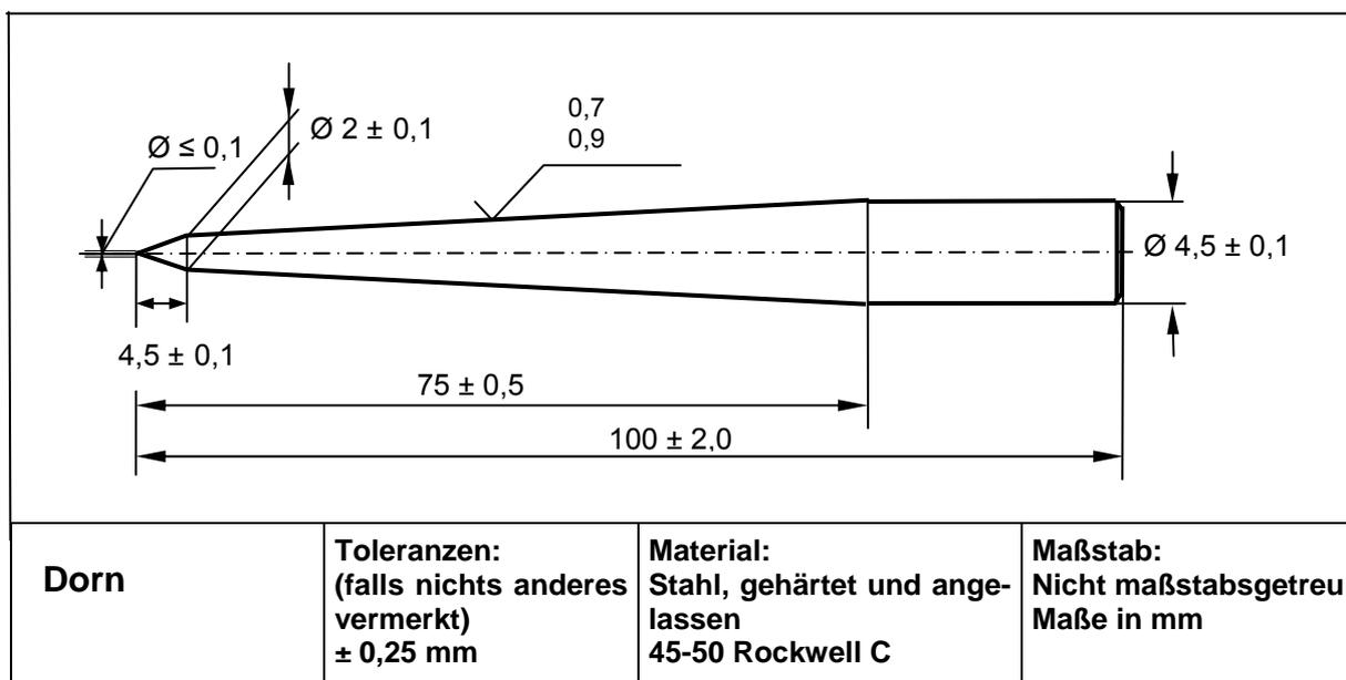
**Hersteller:** Fa. High Speed and Carbide Ltd., England, Engineered Spike PSDB/
